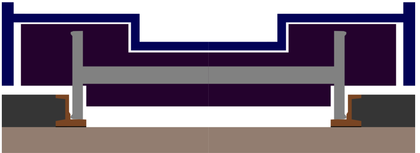
Figure 70: LCRT track with flat rails for flangeless wheels with stiffening braces on the outer side, displayed with wheelset (grey), running gear (violet) and car body (blue).
