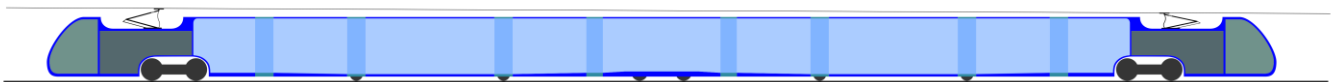
Figure 6: Vehicle version with driven high-floor bogies under the end segments, a driven four-wheel running gear in the middle and a total of four non driven portal wheelsets. In the area of the non-driven portal wheelsets, floor height is 25 cm and inner height is 210 cm, above driven wheels, floor height is 35 cm and inner height is 200 cm.
