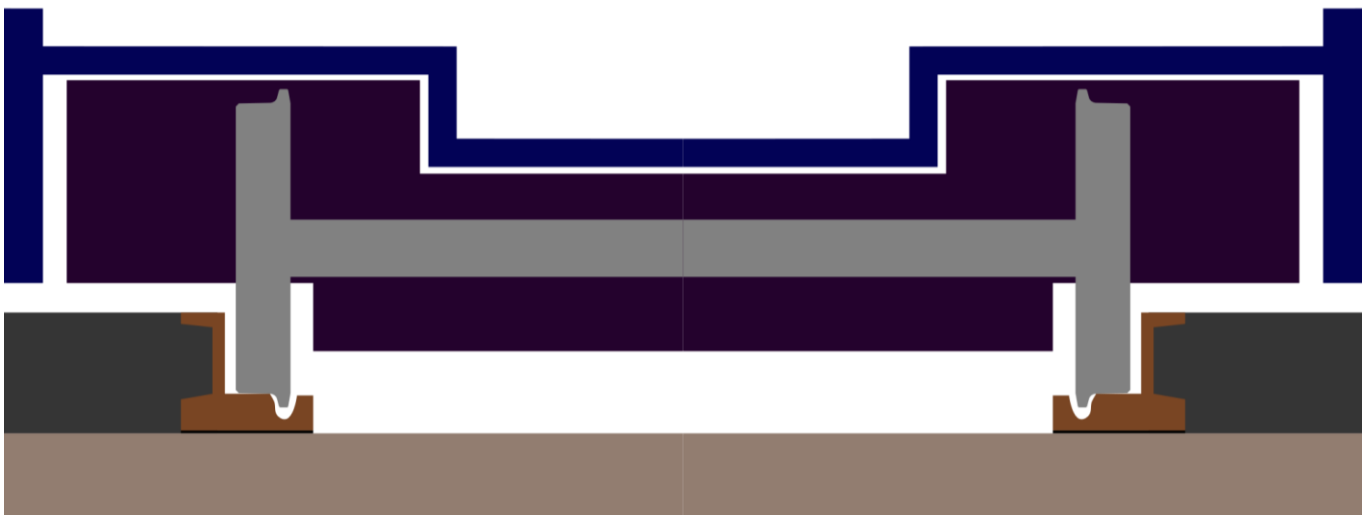
Figure 68: LCRT track with flat rails for flanged wheels with stiffening braces on their outer side, displayed with wheelset (grey), running gear (violet) and car body (blue).
