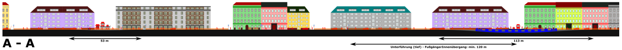
Figure 23: Longitudinal section of an LCRT-Line with a shallow underpass (left part), station area (center) and a deep underpass (right part)
