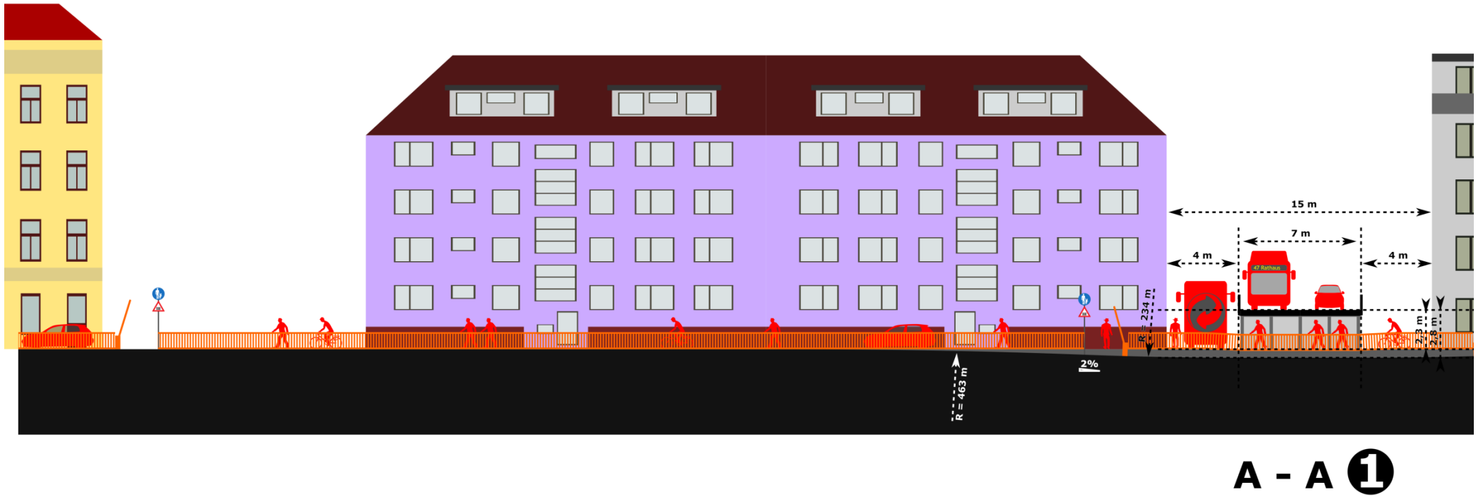
Figure 26: Detailed view of a longitudinal section of an LCRT line in the area of shallow underpass.
