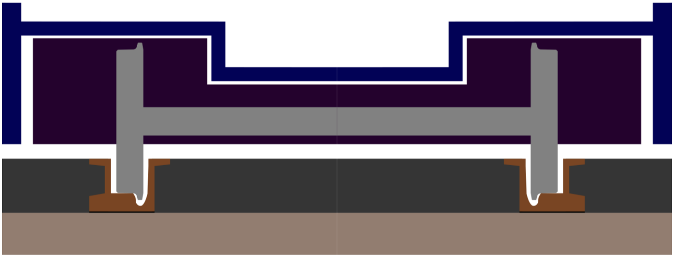
Figure 67: LCRT track with flat rails for flanged wheels with stiffening braces on both sides, displayed with wheelset (grey), running gear (violet) and car body (blue).
