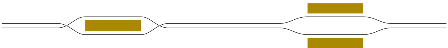
Figure 84: Single-track line for rubber-tyred vehicles with asymmetric guiding rail (modified Translohr system) with two passing loops, one with an island platform and one with side platforms.
