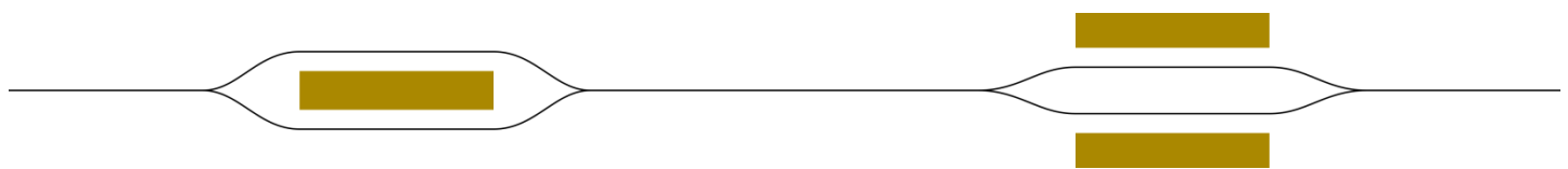
Figure 78: Single-track line for rubber-tired vehicles with central guiding rail (Translohr System) with switches, Overview with two passing loops, one with an island platform and one with side platforms.
