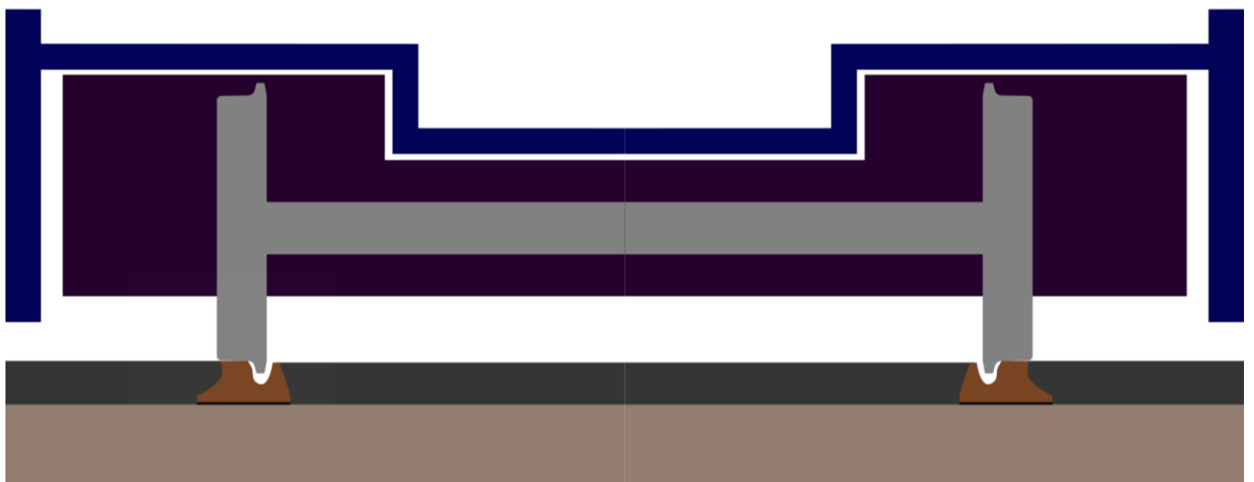
Figure 66: LCRT track with flat rails without any stiffening braces, displayed with wheelset (grey), running gear (violet) and car body (blue).
