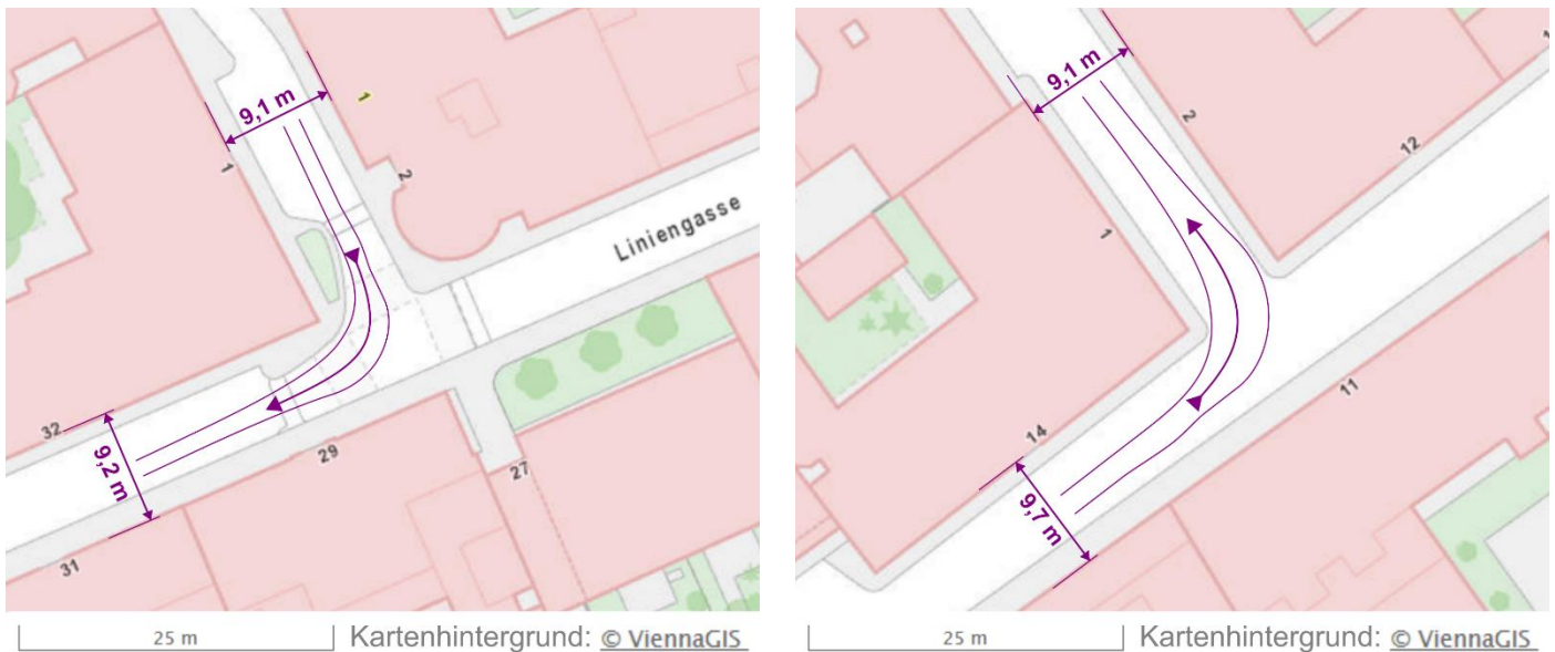
Figure 2: Overlay of the tractrix curve of the car body of a 18 m long and 1,85 m wide bi-articulated minibus over two exemplary street crossings in Vienna: Bürgerspitalgasse / Liniengasse (left) and Liniengasse / Haydngasse (right). The tractrix curves are those of 24,7 m long and 2,55 wide existing bi-articulated bus 2 , downsized by a linear factor of 72,8%.
